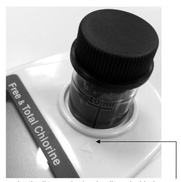
Please make the line on the bottle aligned with the arrow on the meter.
